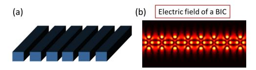
Fig. 1. (a) Schematic of a one-dimensional (1D) photonic crystal membrane, which is also referred to as high-contrast grating (HCG) structure. (b) The electric field profile of an example BIC in the structure.
