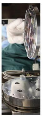
In our team we aim to develop these homostructures towards development of novel quantum devices using a Metalorganic vapour phase epitaxy (MOVPE) reactor. We are actually growing InP NWs by self catalization on Si and InP wafers. To improve crystal purity and achieve phase switching, we are employing different strategies along with feedbacks from electronic microscopy and optical characterization.
