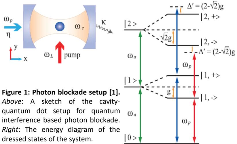
**Figure 1: Photon blockade setup [1].**
