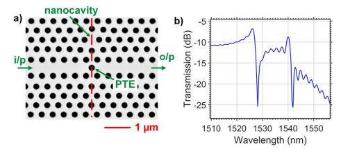
Fig. 1: (a) Scanning electron microscope image of a point defect nanocavity side-coupled to a line-defect photonic crystal waveguide. (b) Finite difference time domain (FDTD) simulated transmission spectrum of the device in part (a).
