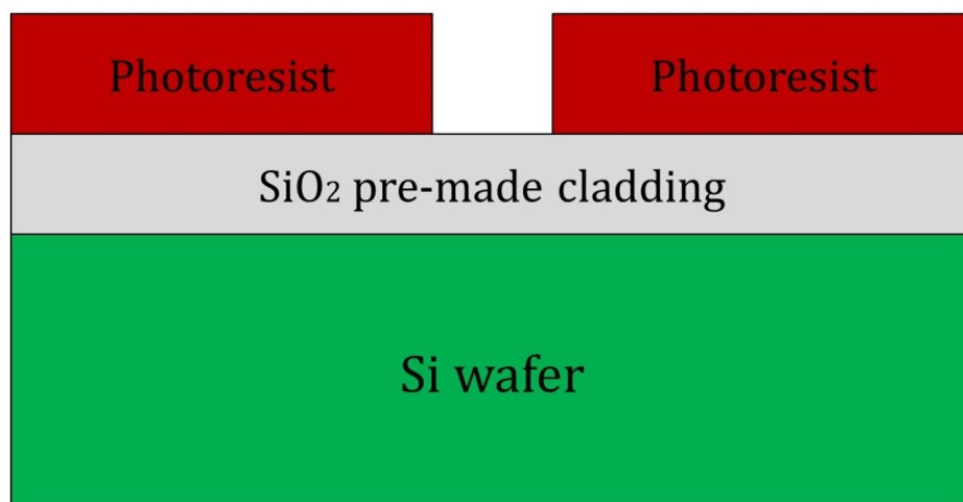
Figure 3.5. Sketch of the wafer after the UV lithography process with the photoresist pattern.
