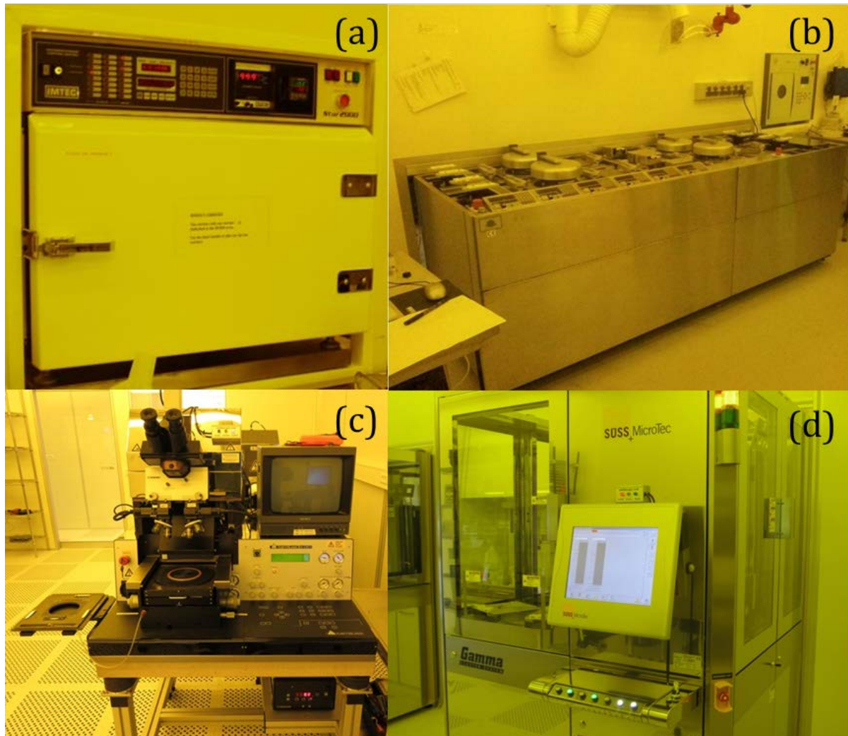
Figure 3.3. Equipment for the UV lithography process: (a) HMDS oven, (b) Spin Track 1+2, (c) KS Aligner, and (d) TMAH UV-lithography Developer.
