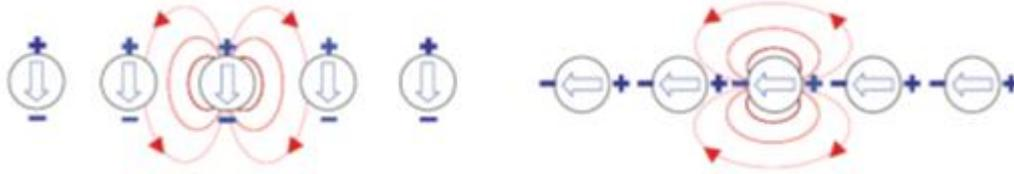
**Figure 2.12:** Schematic of near-field coupling between metallic nanoparticles for the two different polarizations. [25]
