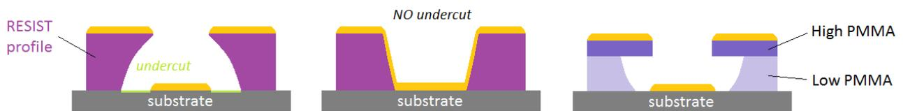
**Figure 4.8:** Illustration of a good lift-off monolayer resist profile (**left**) because of the presence of an undercut; bad resist without undercut, thus preventing lift-off (**centre**); double PMMA resist (**right**), developing at different rate because of different molecular weight (the bottom one has a lower molecular weight).
