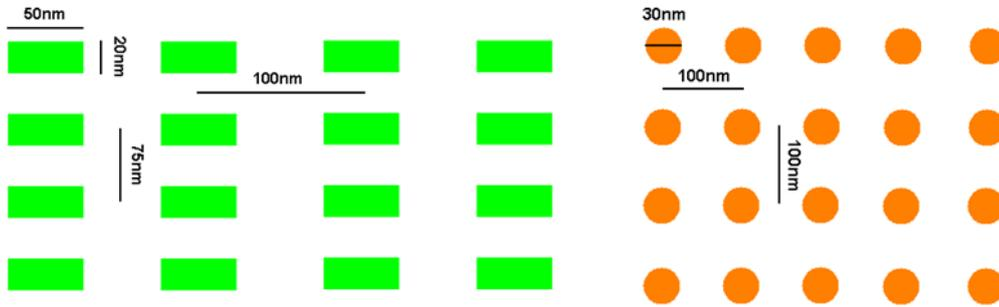
**Figure 4.3:** Draw of the structures that are initially aimed through EBL.
