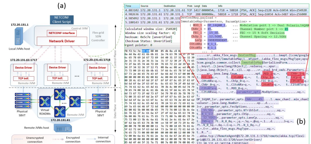
Fig. 5. (a) Demonstration setup (distributed deployment), (b) Device Configuration Message capture
