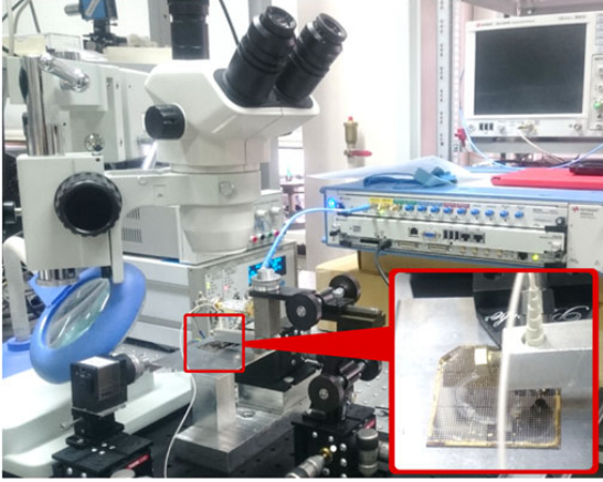
Fig. 3. The precision alignment probe station with SM-VCSEL chip wafer (inset).
