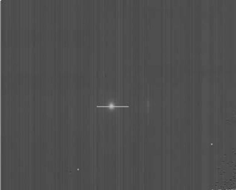
Figure 5.5: Grayscale image showing spontaneous emission when 980 nm pump laser is positioned on top of InP layer with active layers (with no device beneath).
