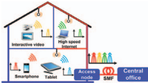
Figure 1 A typical indoor scenario with multiple wireless uplink applications using FDMA scheme. [Color figure can be viewed in the online issue, which is available at wileyonlinelibrary.com ]
