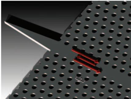
Figure 2.2: Illustration of the forward and backscattering which a slow light mode experiences. The lattice constant,  $a$ , is marked in the figure.
