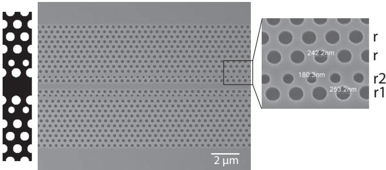
Figure 5.3: Left: a unitcell of the optimized design. Middle: SEM image of the fabricated structure. Right: a magnification showing the size of the holes  $r_1$  at the bottom of the image, followed by  $r_2$  and  $r$ . The location shift of the two rows closest to the waveguide can be seen.
