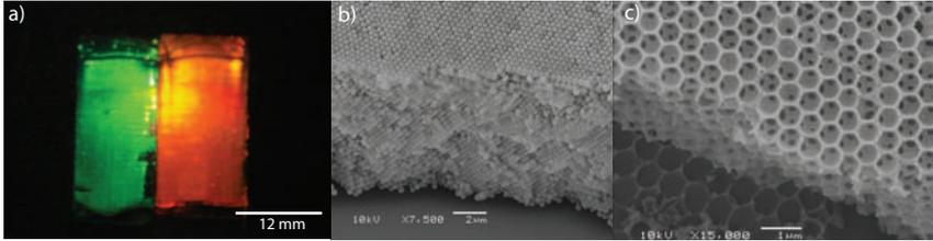
Figure 1.1: a) Photo taken under white light illumination of two polystyrene opals created on microscope slides. To the left: sphere size 270 nm. To the right: sphere size 240 nm. b) SEM image of a polystyrene opal. Showing the long range order also in the third dimension, a thickness of about  $20\mu\text{m}$  achieved in a single growth. c) Sol-gel inverse opal. [20]
