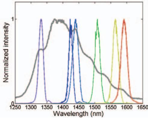
Figure 6.4: ASE spectra (gray) and normalized laser emission spectra at each wavelength at which pump probe measurements were carried out. The wavelengths  $1423, 1440nm$  and  $1565, 1590nm$  correspond to a dip and a peak respectively. The chosen wavelengths covers a range of  $260nm$ .
