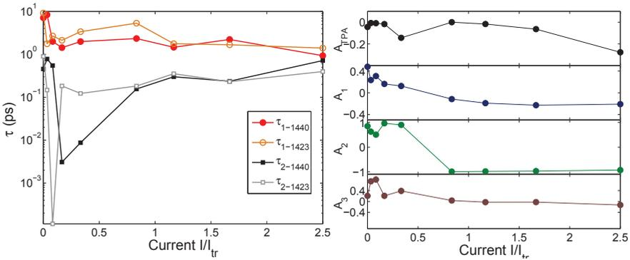
Figure 6.8: Left: Characteristic gain recovery times for QD SOA as a function of injection current. Slow component ( $\tau_1$ ) shown in red and fast component ( $\tau_2$ ) shown in black. Derived time constants for both  $1423nm$  and  $1440nm$  are shown for comparison. Right: normalized amplitudes coefficients (at  $\lambda = 1440nm$ ) of the response function in Eq. 6.3.
