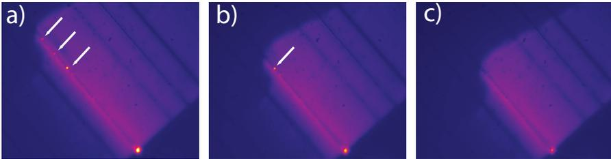
Figure 4.24: A photo series taken with an IR camera while pumping different lengths of a 10 QW sample with three distinct lasing modes in the PhC waveguide. The guided ASE intensity (seen as scattering out of plane at the taper tip at the bottom of each image) is drastically reduced as the lasing modes are shadowed.
