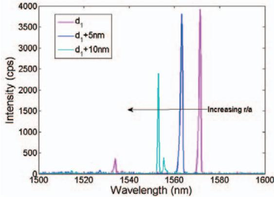
Figure 5.10: Samples:  $70\ \mu\text{m}$  long 3QD lasers of different designs. Pump: RegA, average power 6 mW. Left: Laser emission spectra from three  $70\ \mu\text{m}$  long 3QD lasers with increasing hole size. All with four-hole output mirror and a out-coupling taper. The cavities are optically pumped with the output from the RegA, at an average power of  $1\text{mW}$ .
