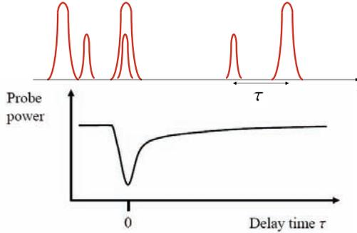
Figure 6.3: A schematic of the delay between the pump (higher amplitude) and the probe (lower amplitude) and the corresponding pump-probe measurement in the gain regime.
