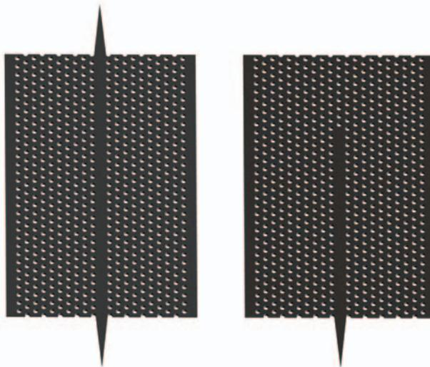
Figure 3.3: An illustration of the two amplifier designs equipped with tapers. Left: an amplifier with input and output tapers. This design can be made down to  $900\mu\text{m}$  long, limited by cleaving capability. Right: an amplifier with one single taper. This design can be made as short as desired.
