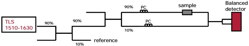
Figure 4.2: An illustration of the MZI set up for dispersion measurements.
