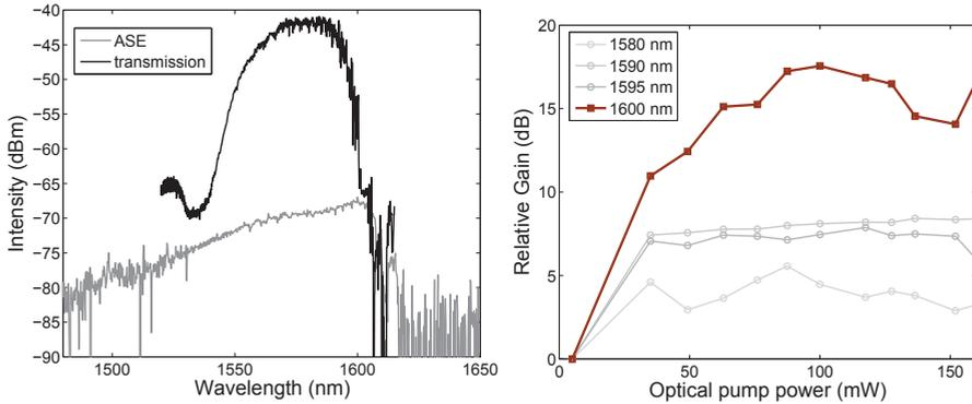
Figure 4.15: Left: ASE (pump: 200mW, 980nm, CW ) and transmission (un-pumped) showing the band edge at 1600nm of the 1 QW sample. Right: Relative gain gain measurement showing highest relative gain in the slow light region. The pump-power levels at the x-axis indicate the peak power of the 500ns long pulses from the 980nm diode.
