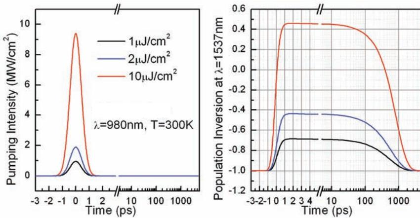
Figure 2.10: Left: An example of short pulse excitation at different energies. Right: the corresponding population inversion at each pump power as a function of time. The time-window for gain is proportional to the carrier lifetime (set to be 500 ps in the calculations). *Figure by courtesy of Yaohui Chen, DTU Fotonik.*
