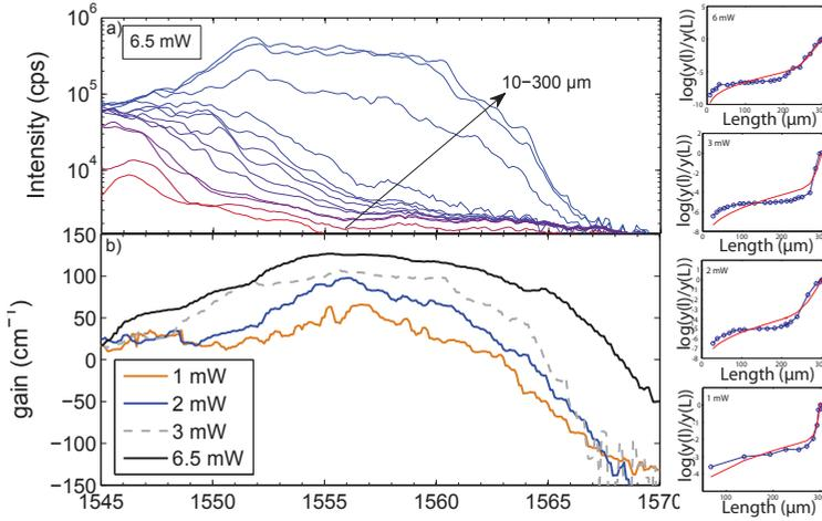
Figure 4.22: Gain extracted from ASE measurements acquired while pumping the different lengths of the  $300\mu\text{m}$  long semi-closed 10 QW PhC waveguide. Data points beyond  $1567\text{nm}$  are not trustworthy as they are beyond the band edge of the guided mode. The legend indicate the average pump powers of the RegA pump. To the right the experimental data along with the fits are presented for each pump power at the wavelength  $1557\text{nm}$ .
