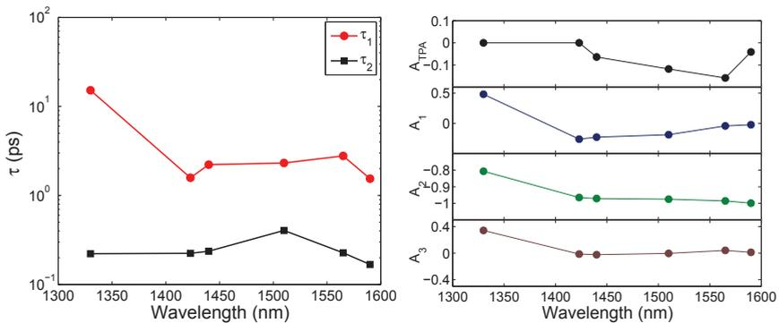
Figure 6.6: Left: Characteristic gain recovery times for QD SOA as a function of wavelength. Slow component ( $\tau_1$ ) shown in red and fast component ( $\tau_2$ ) shown in black. Right: normalized amplitudes coefficients of the response function in Eq. 6.3. The applied current is fixed at  $100mA$ .
