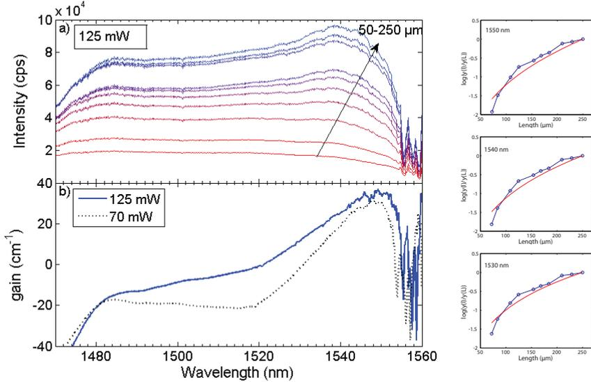
Figure 4.11: Left: a) ASE spectra measured while pumping different lengths of the PhC waveguide (sample B, 1 QW). Pump power 125 mW peak power, pulse duration  $500\text{ns}$ , period  $50\mu\text{s}$ , wavelength  $980\text{nm}$ . b) the extracted gain for 125mW and 70mW pulse peak power. Right: Measured data (blue) and fit (red) for three representative wavelengths (1530, 1540, 1550 nm)
