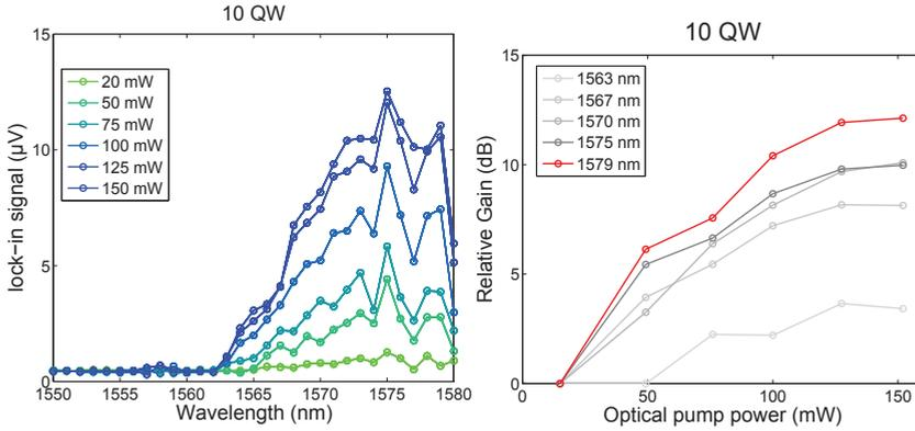
Figure 4.16: Left: Change of transmission for the 10 QW PhC waveguide at several different pump powers. Right: the derived relative gain. The indicated pump-power levels are peak power of the  $500ns$  long pulses from the  $980nm$  diode.
