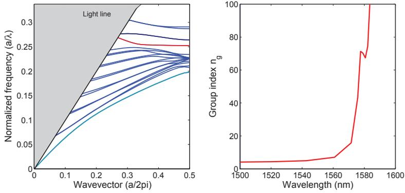
Figure 5.2: Dispersion diagram (left) and group index (right) from a 3D MPB calculation of the optimized design. A lattice constant of  $400\text{nm}$  (membrane thickness  $340\text{nm}$ ) brings the band edge to about  $1580\text{nm}$ .
