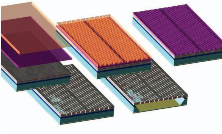
Figure 3.1: An illustration of the processing steps involved to achieve a free-standing membrane PhC.
