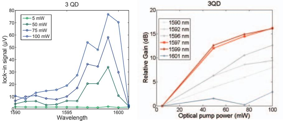
Figure 4.17: Left: Change of transmission for the 3QD PhC waveguide at several different pump powers. Right: the derived relative gain. The indicated pump-power levels are peak power of the  $500ns$  long pulses from the  $980nm$  diode.
