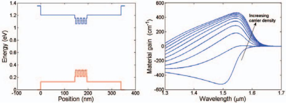
Figure 2.5: Left: Band diagram of the membrane with 4 QWs of  $6\text{nm}$  thickness. The dashed lines in the QW region indicates the lowest quantum confined state (calculated for a single well). The depth of the wells are noted in the legend. Right: Calculated gain curves for carrier densities ranging from  $1 \cdot 10^8 - 30 \cdot 10^{12}$ .
