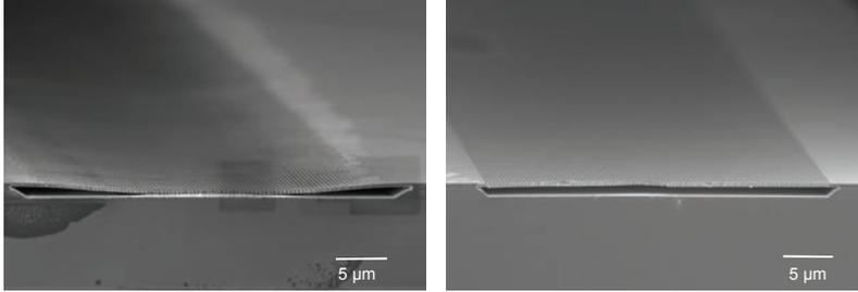
Figure 3.10: Identical samples on a wafer with a  $200nm$  thick InAlAs sacrificial layer, the only difference is the wet etch chemistry. Left:  $H_3PO_4/HCl$  etch. Right:  $HCl : H_2O$  etch.
