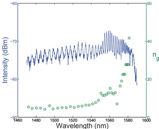
Figure 4.1: Spontaneous emission from a  $50\mu\text{m}$  short PhC waveguide with a hole diameter of  $210\text{ nm}$  and flat end facets (RBW =  $0.1\text{ nm}$ ). The deduced group index is shown in green.
