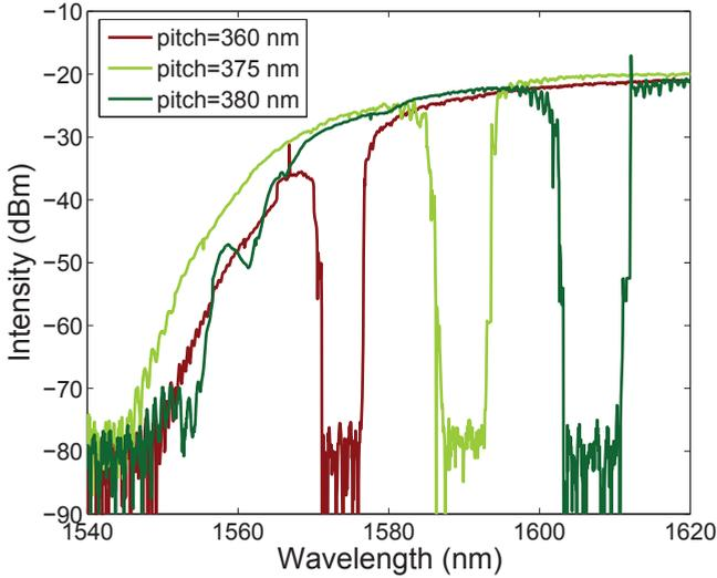
Figure 4.13: Transmission spectra from un-pumped 10 QW waveguides with different lattice constants. The green spectra with  $a = 380\text{nm}$  is measured on Sample C.
