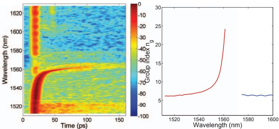
Figure 5.4: Left: time wavelength map of the topology optimized sample. Plotted on a log scale normalized to maximum transmission. Dark red is maximum transmission (0dB). Right: Extracted group index, using the sample length,  $1\text{mm}$ . The mode with zero dispersion at  $1580 - 1600\text{nm}$  is plotted in a different colour because it is believed to be a different mode.
