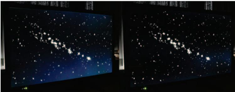
**Figure 2.20:** Displayed results of the Stars image (as in Table 2.7) for backlight algorithm *Albrecht* [36] (left) and gradient descent with no power penalty (*GDq0*, right) [10].
