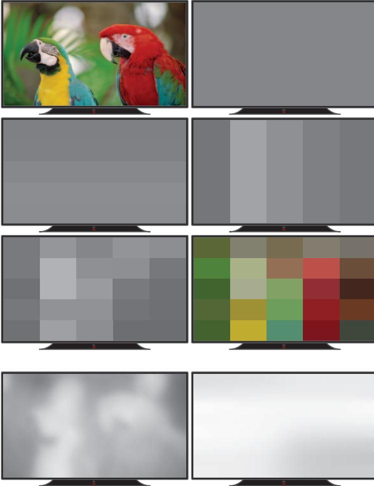
**Figure 2.7:** Examples of backlights depending on the type and position of backlight segments. From top to bottom, left to right: input image, global (0D) backlight, horizontal (1D) backlight, vertical (1D) backlight, 2D backlight, 3D (2D+color) backlight. The two bottom displays are examples of the backlight generated from the input image in case the backlight is 2D direct-lit (left) or edge-lit (right).
