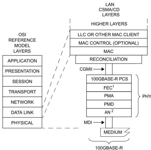
Figure 2.4 - Ethernet Layers (modified from [9]).
