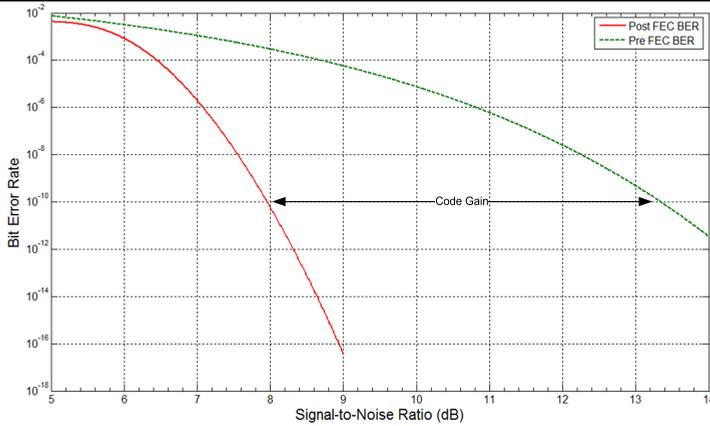
Figure 5.1 – Simulation showing the bit error rate before and after Reed-Solomon FEC decoding as a function of the SNR.
