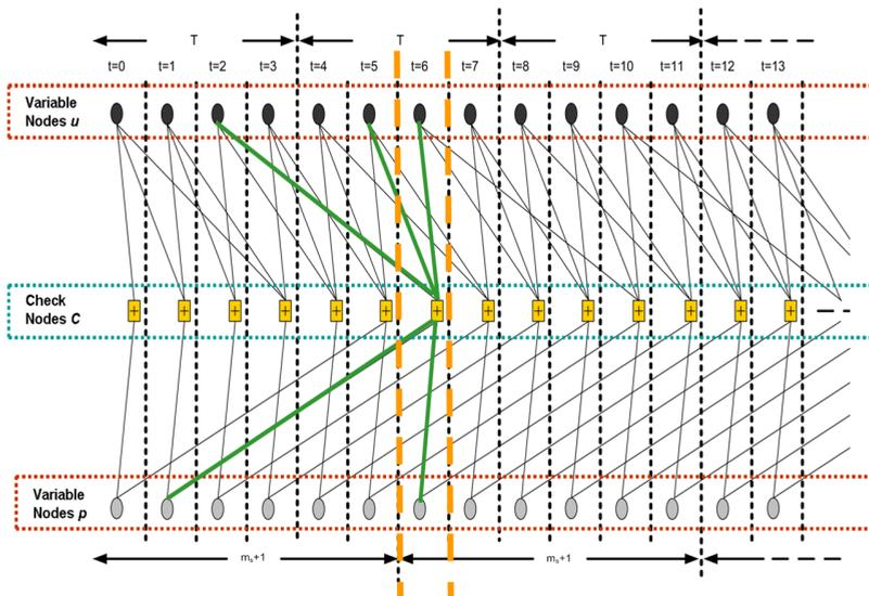
Figure 5.6 - Tanner Graph for rate  $\frac{1}{2}$  (5, 3(2), 5) LDPC-CC time-variant decoder. Each processor deals with a specific  $m_s+1$  part of the graph. Black and grey nodes represents variable nodes with three (3) and two (2) variable degrees respectively and yellow nodes represent check node units with five (5) check degree. [107].
