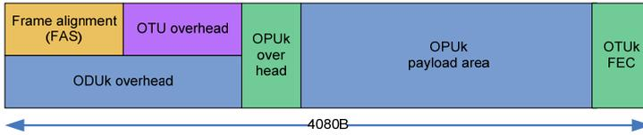
Figure 6.1 – Standard OTN Frame structure (not to scale) [99].
