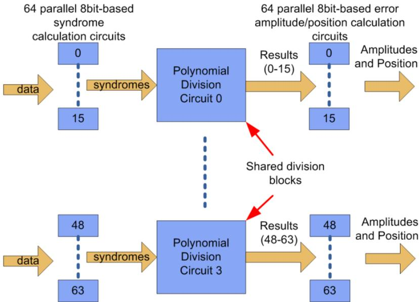
Figure 5.5 – Parallel Reed Solomon decoding circuit.
