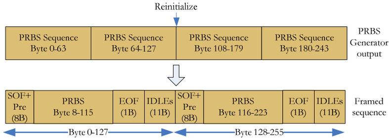
Figure 2.10 - Framing of two adjacent minimum size frames.
