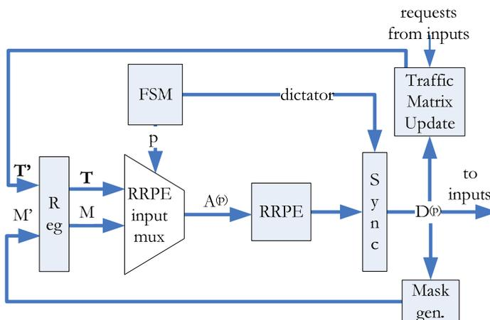
Figure 4.3 - MLRRMS hardware implementation. This scheduler performs look ahead using an iterative approach, where the fan-outs of the packets in the queues are scanned in a sequential manner, incrementing the position pointer  $p$  for each clock cycle.
