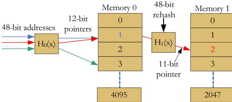
Figure 3.6 – Basic MAHT structure with two tables (memory banks). In event of a collision in table 0, the collided address is rehashed to table 1 using a different hash function. The tables decrease in size ( $N$ ) as  $M$  increases.
