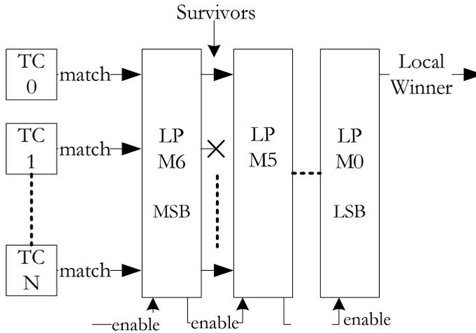
Figure 3.14 - Local LPM circuit for post-processing address mates from  $N$  TCAM rows.
