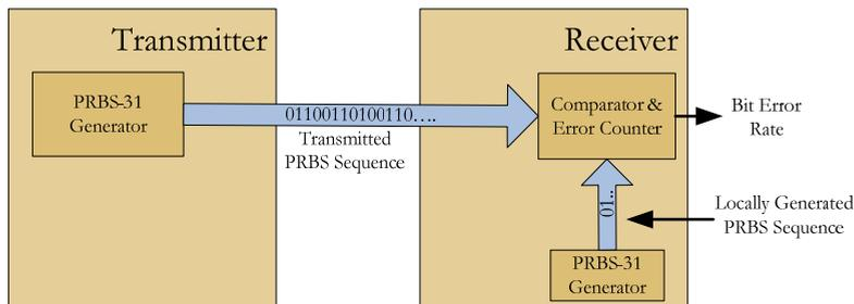
Figure 2.5 - Bit Error Rate Tester (BERT).
