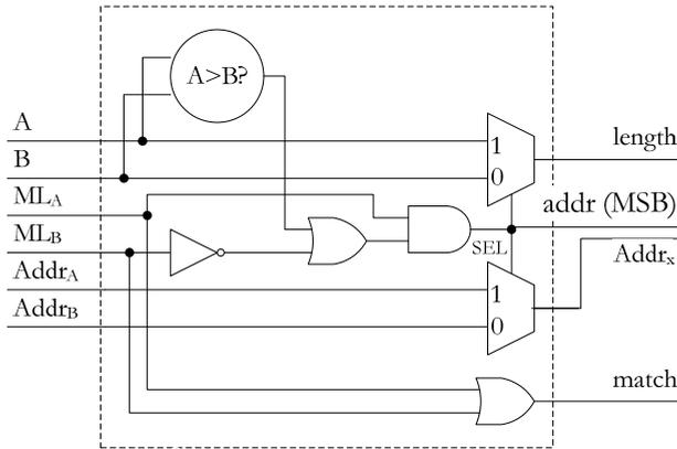
Figure 3.18 - Comparator Element
