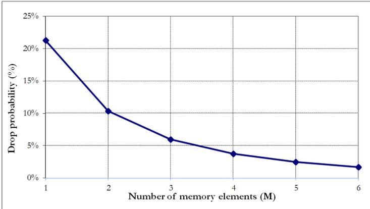
Figure 3.4 –Simulation of the drop probability when storing the same number of MAC addresses in tables with different values of  $M$ , but constant total memory size (the  $N \times M$  product). The load factors for  $M=1..6$  is 50%, 25%, 16.6%, 12.5%, 10% and 8.3%, respectively.
