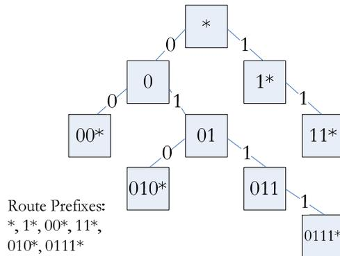
Figure 3.10 – 1-bit trie structure for IP lookup.
