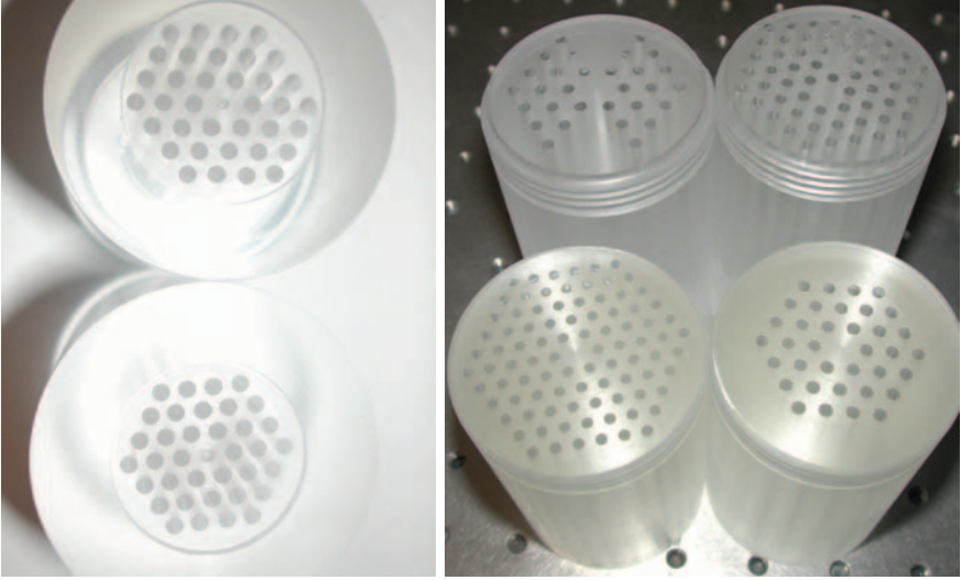
Figure 3.2: Example of PMMA and TOPAS preforms.
