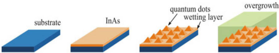
Figure 4.4: Schematic of the growth process of self-assembled QDs in the Stranski-Krastanov mode [19].
