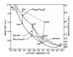
Figure 1.6: Bandgap vs. lattice constant for III-V compounds. The red line indicate the quaternary alloys, InGaAsP, lattice matched to InP [34].
