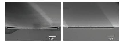
Figure 3.10: Identical samples on a wafer with a 200nm thick InAlAs sacrifical layer, the only difference is the wet etch chemistry. Left:  $H_3PO_4/HCl$  etch. Right:  $HCl: H_2O$  etch.
