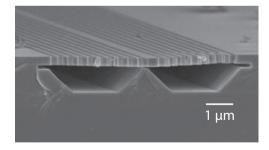
Figure 3.8: Two samples with different InAlAs thickness. Left: 800 nm. Right: 50 nm.
