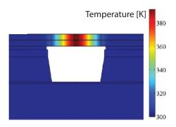
Figure 2.9: Numerical simulation results for a vertical cross section of the InGaAsP membrane structure. Figure by courtesy of Luca Carletti, DTU Fotonik.
