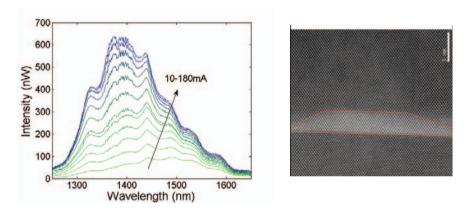
Figure 6.1: Left: ASE spectrum from an electrically biased 5QD SOA at currents ranging from 10 to 180 mA. (RBW=2nm) Right: HAADF STEM image of a GaAs capped InAs QD followed by InGaAsP. The InAs rich dot appear bright in the image, red lines are guides to the eyes. Figure by courtesy of Shima Kadkhodazadeh, DTU Fotonik.
