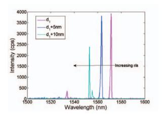
Figure 5.10: Samples: 70  $\mu$ m long 3QD lasers of different designs. Pump: RegA, average power 6 mW. Left: Laser emission spectra from three 70 $\mu$ m long 3QD lasers with increasing hole size. All with four-hole output mirror and a out-coupling taper. The cavities are optically pumped with the output from the RegA, at an average power of 1mW.
