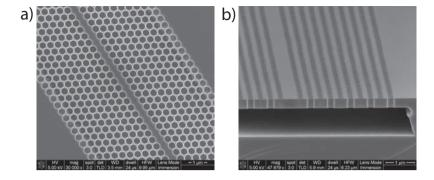
Figure 1.3: SEM image of 2D membrane PhC. a) Top view showing the linear waveguide defect. b) Sideview of a cleaved facet showing the free-standing membrane surrounded by air, for efficient confinement in the third dimension.
