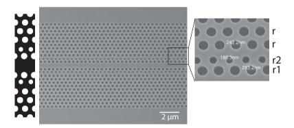
Figure 5.3: Left: a unitcell of the optimized design. Middle: SEM image of the fabricated structure. Right: a magnification showing the size of the holes  $r_1$  at the bottom of the image, followed by  $r_2$  and r. The location shift of the two rows closest to the waveguide can be seen.
