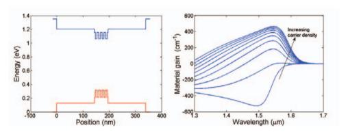
Figure 2.5: Left: Band diagram of the membrane with 4 QWs of 6nm thickness. The dashed lines in the QW region indicates the lowest quantum confined state (calculated for a single well). The depth of the wells are noted in the legend. Right: Calculated gain curves for carrier densities ranging from  $1 \cdot 10^8 - 30 \cdot 10^{12}$ .
