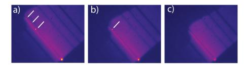
Figure 4.24: A photo series taken with an IR camera while pumping different lengths of a 10 QW sample with three distinct lasing modes in the PhC waveguide. The guided ASE intensity (seen as scattering out of plane at the taper tip at the bottom of each image) is drastically reduced as the lasing modes are shadowed.
