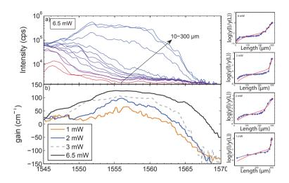
Figure 4.22: Gain extracted from ASE measurements acquired while pumping the different lengths of the  $300\mu m$  long semi-closed 10 QW PhC waveguide. Data points beyond 1567nm are not trustworthy as they are beyond the band edge of the guided mode. The legend indicate the average pump powers of the RegA pump. To the right the experimental data along with the fits are presented for each pump power at the wavelength 1557nm.
