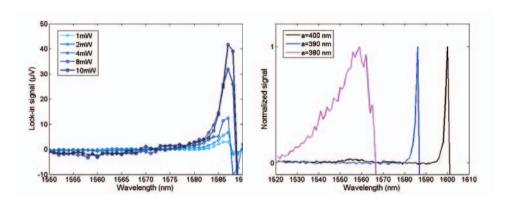
Figure 4.20: Left: Change of transmission at several different pump powers, average power of the RegA pump noted in the legend. Sample: 10 QW semi-closed (sample D) Right: lock-in measurements on 10 QW samples with different lattice constants, each normalized with its peak value. A high transmission correlate with the slow light region of each crystal.
