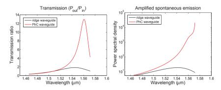
Figure 2.7: Transmission (left) and ASE (right) with and without slow down factor.
