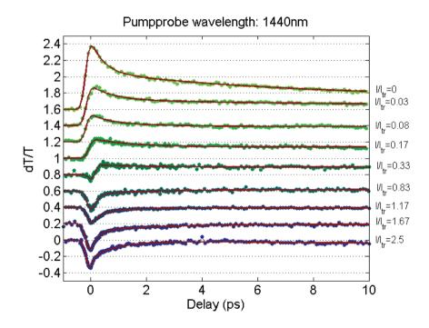
Figure 6.7: Differential transmission at  $\lambda = 1440nm$  as a function of injected current. The different colours green to blue indicate increasing current, as indicated relative the transparency current  $(I_{tr} = 60mA)$  in the border. Each curve is offset 0.2 for clarity. Solid red lines represents the fitted response function to each measurement.
