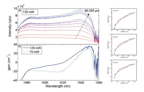
Figure 4.11: Left: a) ASE spectra measured while pumping different lengths of the PhC waveguide (sample B, 1 QW). Pump power 125 mW peak power, pulse duration 500ns, period  $50\mu s$ , wavelength 980nm. b) the extracted gain for 125mW and 70mW pulse peak power. Right: Measured data (blue) and fit (red) for three representative wavelengths (1530, 1540, 1550 nm
