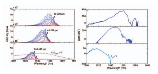
Figure 4.23: Gain measurements on three 10 QW PhC waveguides with different lattice constants. All are pumped with RegA at an average power of 6 mW. a-b) PhC waveguide with lattice constant 380nm (Sample C). c-d) PhC waveguide with lattice constant 375nm. e-f)PhC waveguide with lattice constant 370nm.
