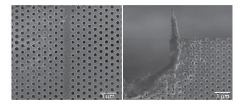
Figure 4.5: SEM images of 1 QW PhC waveguides, each during experiments. Left: burned when pumping CW with 300mW, 980nm from the top. Right: burned when coupling CW 2mW, 1550nm onto the in-coupling taper.
