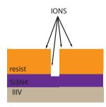
Figure 3.6: An illustration of the shadowing effect. The etch rate is reduced if the ions have limited access to the etch surface.
