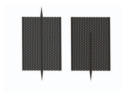
Figure 3.3: An illustration of the two amplifier designs equipped with tapers. Left: an amplifier with input and output tapers. This design can be made down to  $900\mu m$  long, limited by cleaving capability. Right: an amplifier with one single taper. This design can be made as short as desired.
