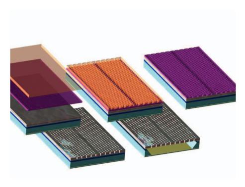
Figure 3.1: An illustration of the processing steps involved to achieve a free-standing membrane PhC.
