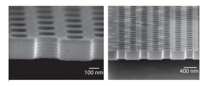
Figure 3.9: Left: SEM image at high magnification showing the debris on the top surface, created in the wet etch of the 200nm thick InAlAs sacrifical layer. The lines in the membrane are the active layers. Right: SEM image showing the surface condition of the same sample after a 150s dip in KOH.
