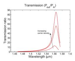
Figure 2.6: Transmission spectra for a PhC amplifier at three different current densities.
