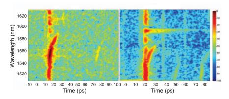
Figure 4.3: Time-wavelength map of two 1 QW waveguides. The colour code is normalized to the highest transmission. Dark red indicates 0 dB while dark blue indicates 100 dB. Left; lattice constant 400nm and hole diameter 210nm, the same design as sample A (Section 4.3.1). Right; lattice constant 400nm and hole diameter 225nm. The dispersive region moves 20nm in wavelength for the larger hole size, as expected.  $(15ps \rightarrow n_q = 4.5 \text{ and } 28ps \rightarrow n_q = 8.4)$
