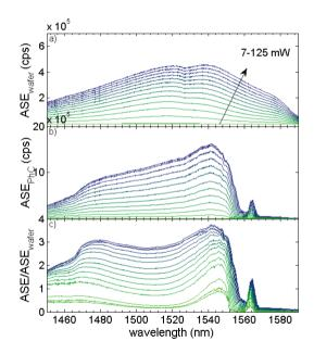
Figure 4.8: a) ASE spectra from the 1 QW wafer at CW pump powers ranging from 7-125 mW (980 nm) b) ASE spectra from sample B c) The normalized ASE, showing the PhC dispersion influence on the spectral shape and an enhancement in the slow light regime. (cps = counts per second)
