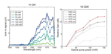
Figure 4.16: Left: Change of transmission for the 10 QW PhC waveguide at several different pump powers. Right: the derived relative gain. The indicated pump-power levels are peak power of the 500ns long pulses from the 980nm diode.
