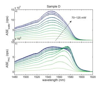
Figure 4.18: ASE spectra from the wafer and  $200\mu m$  long semi-closed sample D respectively (10 QW). Pump: 980 nm diode, CW at powers ranging from 7-125 mW.
