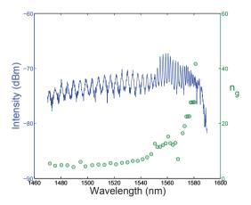
Figure 4.1: Spontaneous emission from a  $50\mu m$  short PhC waveguide with a hole diameter of 210 nm and flat end facets (RBW= 0.1 nm). The deducted group index is shown in green.
