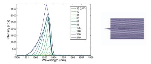
Figure 5.9: Left: emission spectra from a 70  $\mu$ m long 3QD laser, pumped by the output from the RegA, the average power is noted in figure. Right: an illustration of the cavity configuration. Four-holes placed in the line defect close to the out-coupling taper forms a partly reflective mirror.
