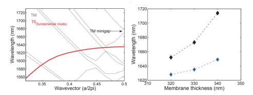
Figure 2.4: Left: dispersion diagram for TM polarization (gray) and the TE fundamental mode (red) (a=400 nm, t=330 nm, r=100 nm). The TM minigap is indicated in the figure. Right: Spectral position of the TE bandedge (blue) and TM minigap (black).
