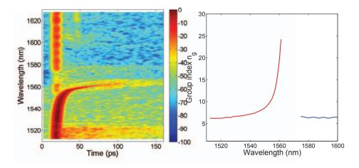
Figure 5.4: Left: time wavelength map of the topology optimized sample. Plotted on a log scale normalized to maximum transmission. Dark red is maximum transmission (0dB). Right: Extracted group index, using the sample length, 1 mm. The mode with zero dispersion at 1580 - 1600nm is plotted in a different colour because it is believed to be a different mode.
