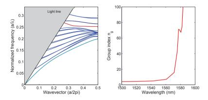
Figure 5.2: Dispersion diagram (left) and group index (right) from a 3D MPB calculation of the optimized design. A lattice constant of 400nm (membrane thickness 340nm) brings the band edge to about 1580nm.
