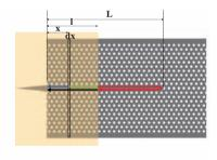
Figure 4.21: An illustration of the semi-closed waveguide, and the pumping scheme used to extract gain and absorption.
