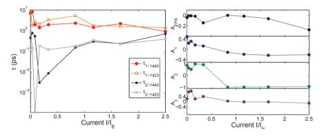
Figure 6.8: Left: Characteristic gain recovery times for QD SOA as a function of injection current. Slow component  $(\tau_1)$  shown in red and fast component  $(\tau_2)$  shown in black. Derived time constants for both 1423nm and 1440nm are shown for comparison. Right: normalized amplitudes coefficients (at  $\lambda = 1440nm$ ) of the response function in Eq. 6.3.
