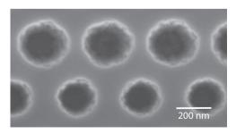
Figure 3.5: SEM image of a bad example of etched holes with very rough edges. The roughness is a result a damaged resist, causing non-perfect holes in the hard mask.
