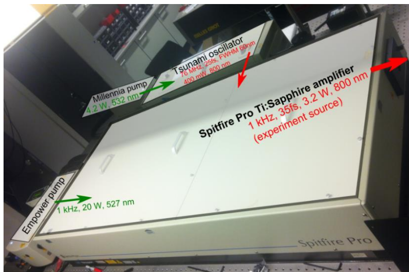
Figure 3.11: Spitfire Pro Ti:Sapphire regenerative amplifier system from Spectra-physics. Reprinted 118
