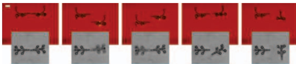
Figure 5.12. Snapshots of simultaneous optical manipulation of two microstructure. The top row shows the images recorded from the side view and the bottom row shows images recorded through the top view. (Figure adapted from [25]).
