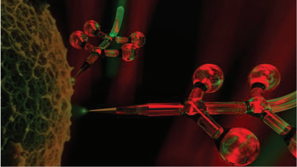
Figure 1.3. Free standing wave-guide microtools that could potentially deliver highly focused light into specific regions within a cell. (Figure adapted from [25]).
