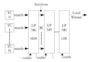
Figure 3.14 - Local LPM circuit for post-processing address mates from NTCAM rows.
