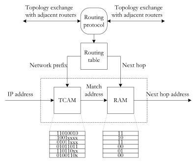
Figure 3.12 - Example of a TCAM-based IP forwarding engine [76].
