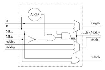
Figure 3.18 - Comparator Element
